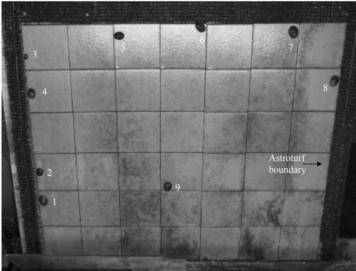
Figure 2.1. Laboratory Setup. Nine Lottia gigantea were placed on a 1 m 2 arena composed of unglazed terra cotta tiles. The numbers were the identifiers for each individual. The dump tank was located above the setup. The dump tank splashed the limpets with water at a regular interval, mimicking the high tide. The dump tank ran for four hours, twice a day. One tile side=15.24 cm
